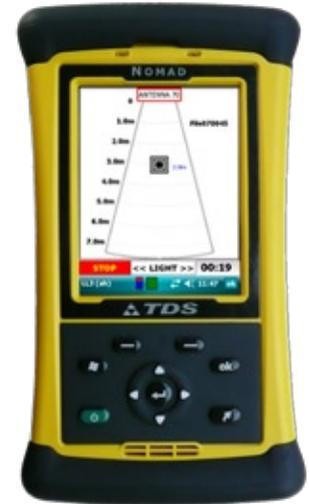
*PDA with black square indicating strong motion detection at 3 meters from sensor.*
