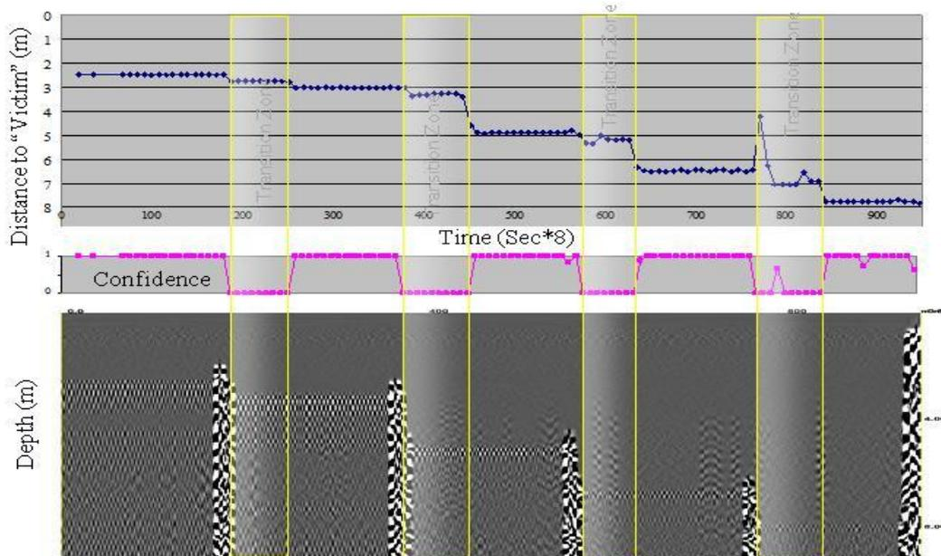
**Figure 3.** Upper plot shows the breathing detection distance vs. time. Note a detection lag of about 10 seconds even after the target has moved his chair further away. Lower plot shows detection confidence between 0 and 100%.
