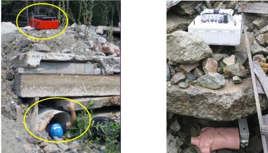
**Figure 5.** Different test in debris piles around the world can only simulate the conditions one might find in an actual emergency. These tests in debris piles used to train dog sniffing teams. The “breathing dummy” was helpful in repeatability testing. The device could successfully detect breathing in both locations.
